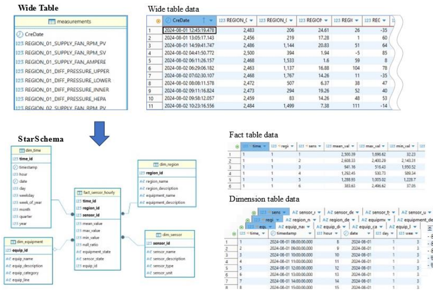
Figure 2. Schema transformation from a wide-table format to a star schema for industrial IoT sensor data.
